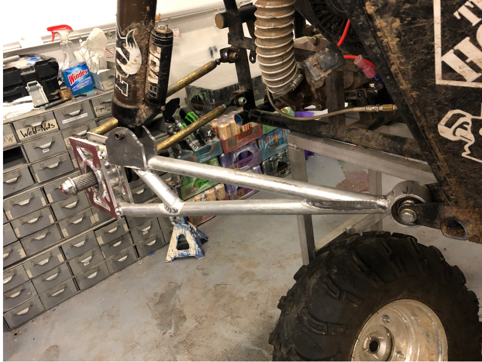
Figure 7. Completed trailing arm for prototype testing
