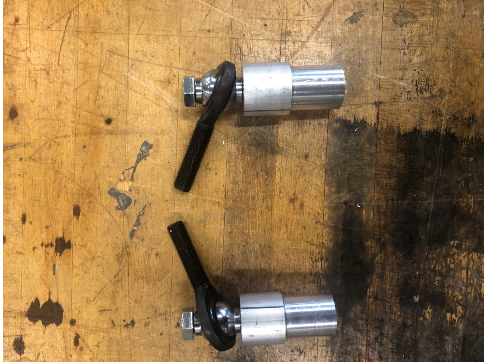
Figure 5. Plugs for end of trailing arm tubing to connect rear lateral links
