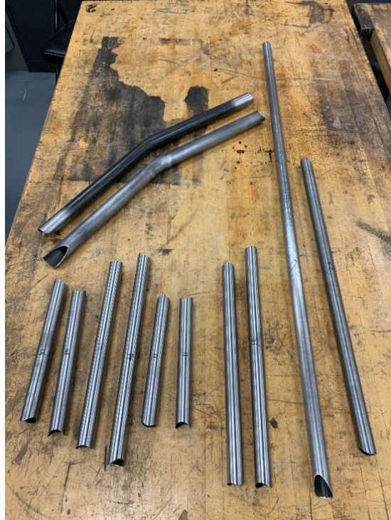
Figure 12. Unwelded frame members
